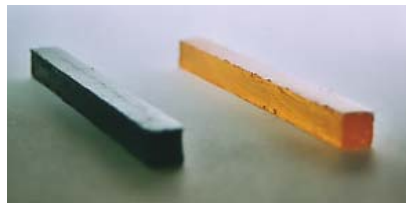
Figure 3.3.8: samples directly produced by RP Left: resin + micro powders of graphite Right: only resin
