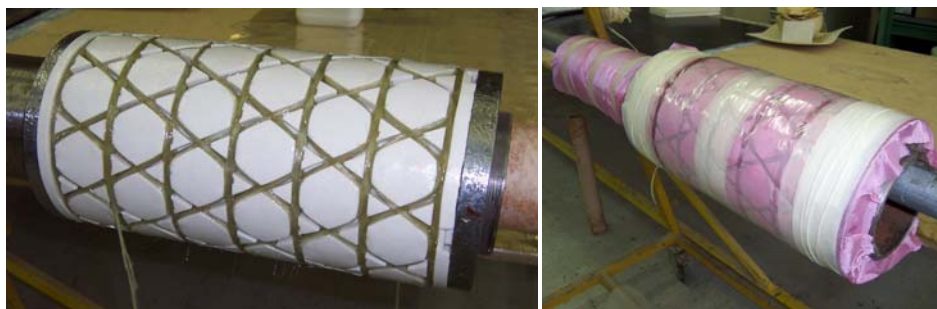
Figure 2.2.3: cylindrical anisogrid lattice structure prototype manufacture
