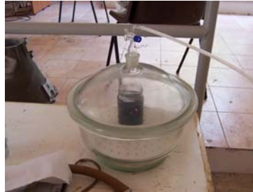
Figure 3.3.1: degassing phase of the resin employed to the manufacturing of micro and nanostructured composite samples by direct Stereo Lithography
