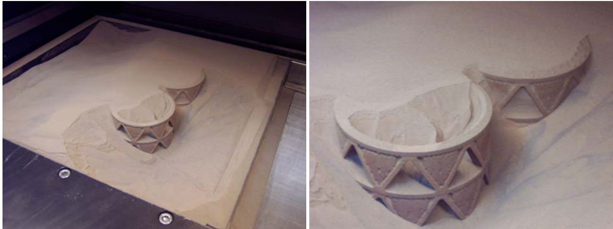
Figure 4.5: the produced isogrid lattice prototypes immersed in the bronze powders
