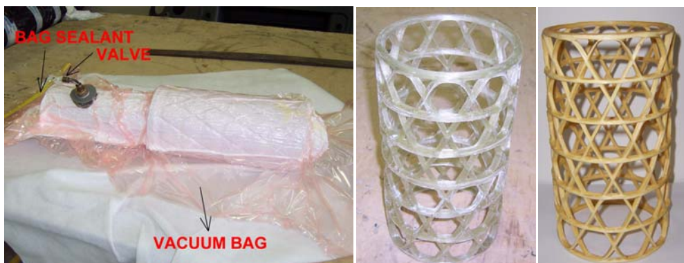
Figure 2.2.4: cylindrical anisogrid lattice structure prototype manufacture
