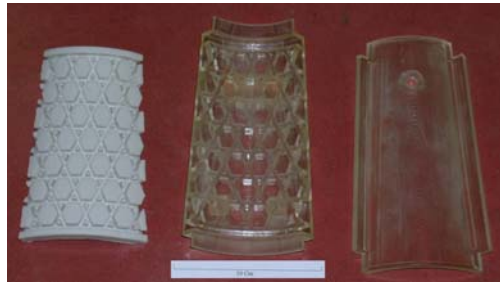
Figure 2.1.7: positive and negative moulds of the conical anisogrid lattice structure prototype
